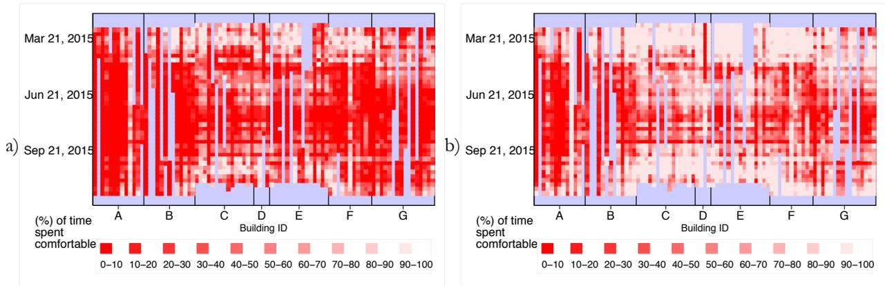
**Figure 1** (a) lower bound of occupant thermal comfort in % of time spent comfortable and (b) upper bound of occupant thermal comfort in % of time spent comfortable. Each square represents an average value in a unit for a week. Gaps in the heat map, where the light blue background is visible, are due to participants withdrawing from the study or entering into the study later than the original date.
