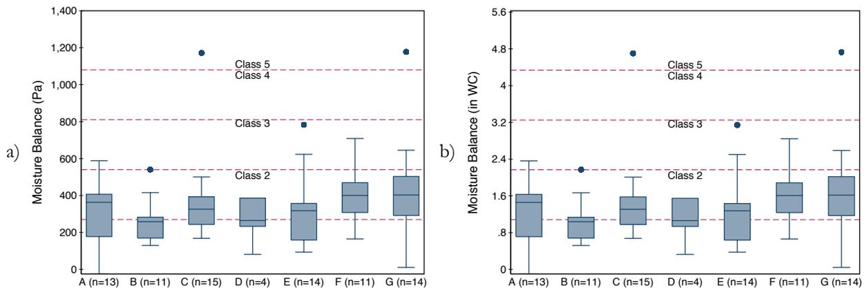
**Figure 4** Moisture balance results for all 7 buildings a) Pa, b) inWC. The moisture balance was determined as the average VPE at all exterior temperatures less than the exterior temperature at inflection. The red dash lines indicate the ISO Standard 13788 indoor climate class. The box plot shows the building median (line), the upper and lower quartiles (upper/lower boundaries of the box), and 1.5· the interquartile range. Dots represent single suite outliers.
