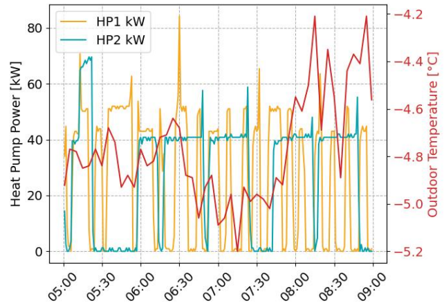
Figure 25. When both heat pumps operated in parallel shorter cycles (here on HP1) were observed.
