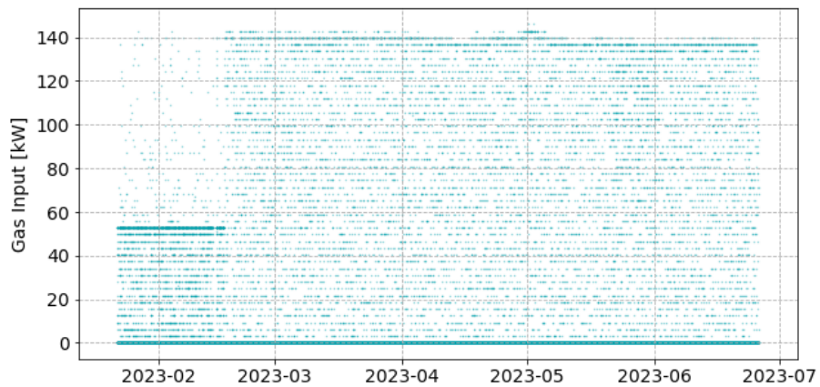
Figure 7. The boiler was on at maximum capacity more frequently after the stepwise change in GHP utilization. Previously it tended to settle on a value less than 60 kW and seldom reached above 140 kW. STEP did not verify why it had previously been settling below 60 kW.
