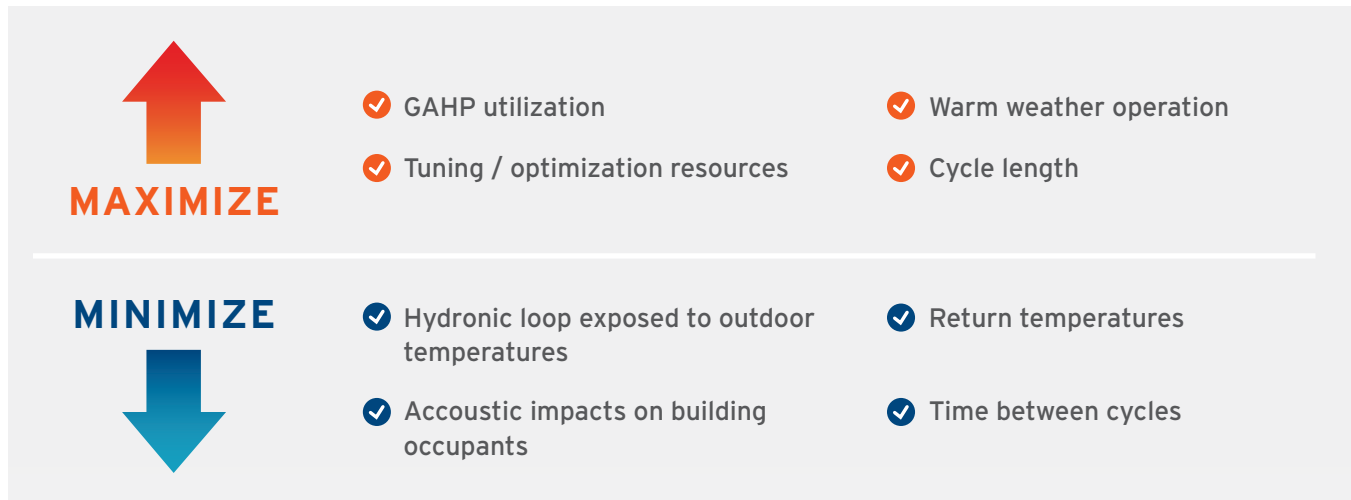
Figure 11: GAHP design and operation considerations
