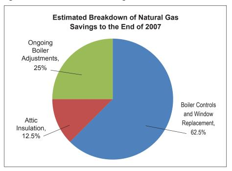
these changes to system operation were made. Also insulation of attic improved the thermal resistance of the building envelope so that set points could be reduced while maintaining a more comfortable temperature. Based on the above allocation, the estimated savings attributed to each retrofit measure is shown in Figure 4.
