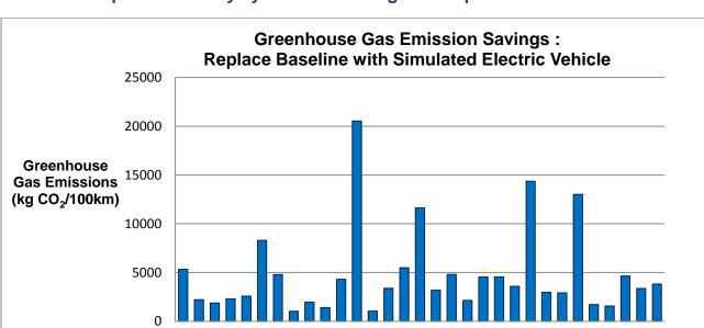
Figure 26: Magnitude of greenhouse gas emission reduction if simulated electric vehicles completed the duty cycle of baseline gasoline-powered vehicles
