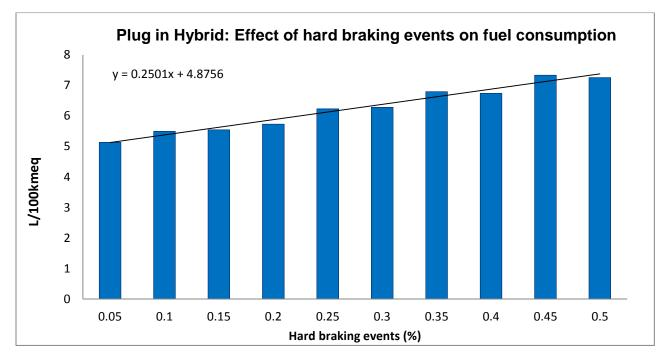
The slopes of the lines in Figures 16 and 17 indicate that fuel consumption per kilometre increases as the percentage of hard acceleration and hard braking increases. Also, these results suggest that hard acceleration had a slightly greater impact at increasing fuel consumption per kilometre than hard braking for plug-in hybrids.
