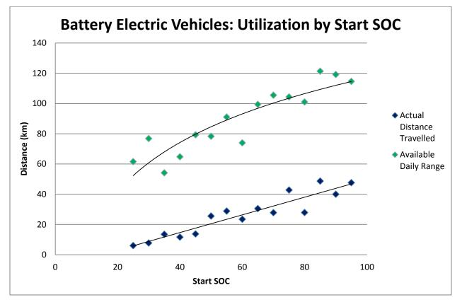
Another finding from Figure 24 is that despite bulk charging, battery electric vehicles are only utilized a fraction of their total available range. The average gap between how far a battery electric vehicle travels each day, and the electric range available was found to be approximately 70 km in this sample.
