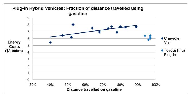
Figure 35: The fuel cost implications of operating plug-in hybrid vehicles without maximizing all-electric range
