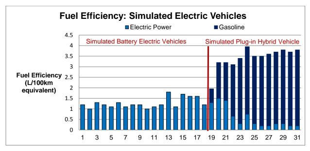
While using plug-in hybrid vehicles increases fuel consumption relative to all-electric vehicles, plug-in hybrids still achieved 57% improvement on average over baseline vehicles. The battery electric vehicles improved fuel consumption by 88%, on average.
