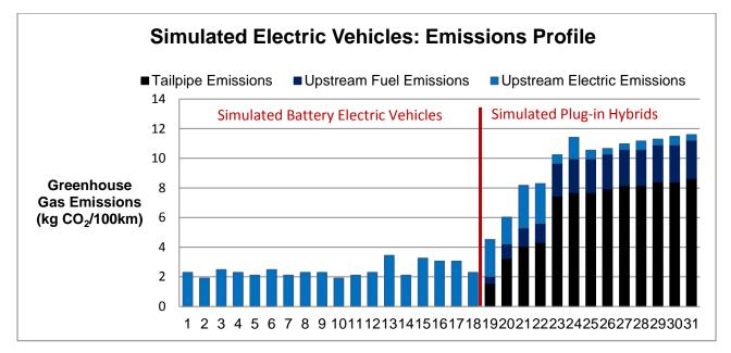
The emissions profile of the simulated vehicle fleet can be broken into the emissions from battery-electric vehicles, and those of plug in hybrids. The greenhouse gas emissions from battery electric vehicles are limited to upstream electricity emissions from power generation and distribution. These emissions are comparatively low from electric vehicles due to their efficient powertrains and the relatively clean electricity grid in Ontario.
