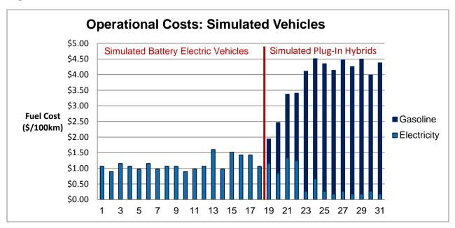
Figure 31: Breakdown of the sources of fuel cost for simulated vehicles
