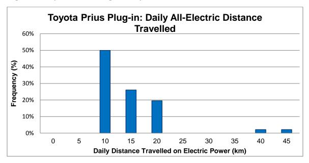
Figure 9: Toyota Prius Plug-in daily all-electric utilization distribution
