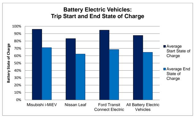
The state of charge values displayed here are the percentage of the usable battery capacity that is available.
