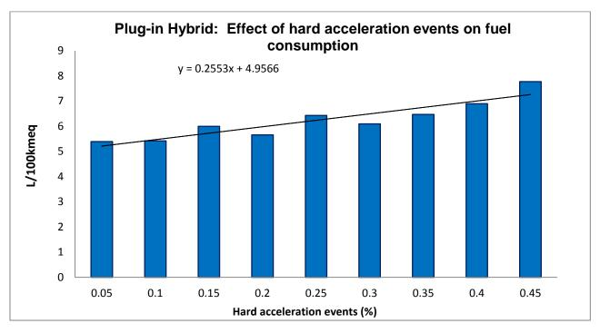
Figure 16: Effect of hard acceleration on fuel consumption of plug-in hybrids
