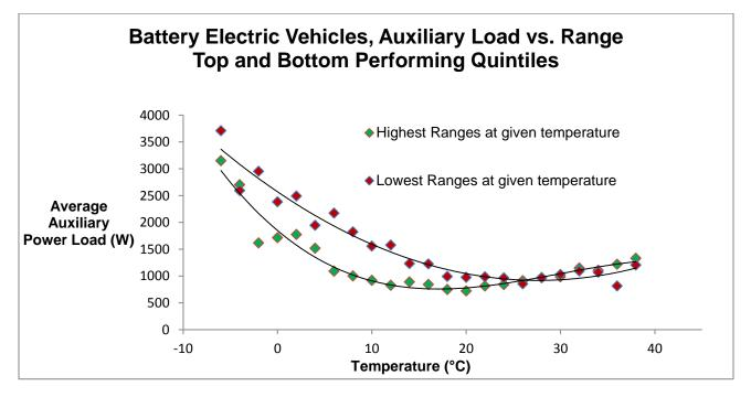
Figure 13: The average auxiliary load between the top and bottom performers of battery electric vehicles
