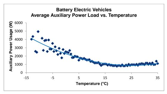
The relationship between auxiliary power usage and temperature indicates that auxiliary power usage is a significant component in the loss of available range at high or low temperatures. As with the temperature and range plot, the effect of auxiliary power usage is much more pronounced at colder temperatures than warmer temperatures.
