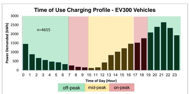
Figure 24: Electric vehicle charging profile throughout the day
