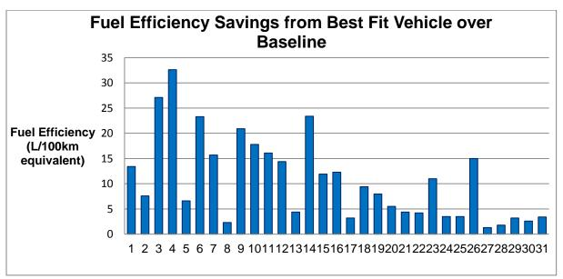
Further inspection of the fuel used by the Best Fit electric vehicles shows the difference in fuel usage between the battery electric vehicles and plug in hybrid vehicles recommended.
