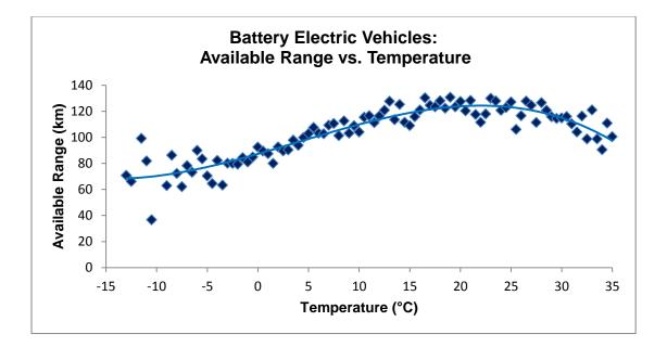
From Figure 10 we can see that the average range a battery electric vehicle has available varies according to the ambient temperature outside. Colder temperatures (those below 15 °C) have a greater impact on range than warmer temperatures (those above 25 °C).
