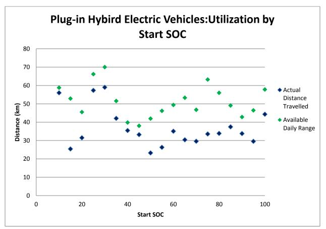
Figure 23: Daily utilization of plug-in hybrids relative to their start of day SOC
