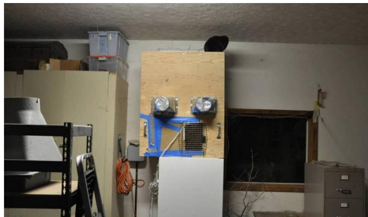
Figure 45: Head-on View of Indoor Unit Test Enclosure
