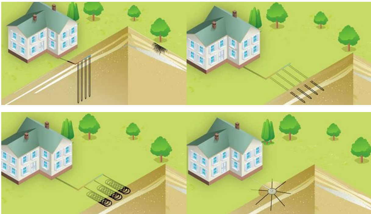
Figure 7: Vertical Loop Field (top left), Horizontal Loop Field (top right), Pond or Lake Loop Field (bottom left) and DX Copper Loop Fields (bottom right) 12
